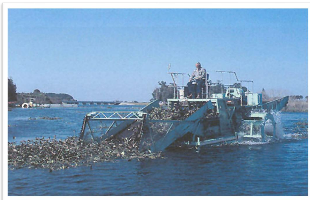
Fig 5: Harvester collecting Water Hyacinth
